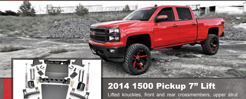
Lifted knuckles, front and rear crossmembers, upper strut spacers, brake line brackets, differential drop brackets, CV spacers, sway-bar drop brackets, lower skid plate, N2.0 Shocks, 6.5" fabricated anti-wrap lift blocks, u-bolts, and brake line bracket.
